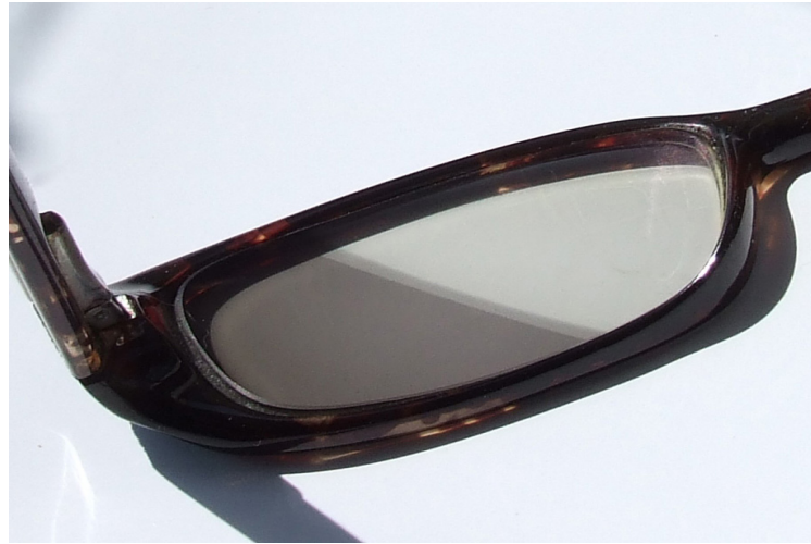
Figure 5: Photochromic lens partially exposed to sunlight
